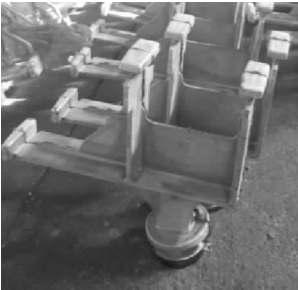
图 4 挤压铸造屏蔽罩支撑铸件毛坯 Fig.4 Squeeze casting shield covers support blanks
