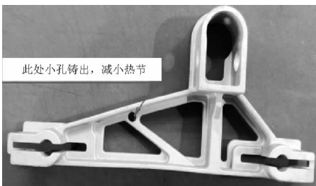
图 1 铸出孔减小热节 Fig.1 Hole by casting to reduce the hot spot
