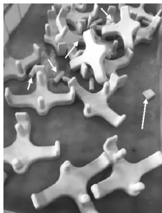
图 6 脱蜡后陶瓷芯断裂 图 7 X 光探伤发现陶瓷芯断裂 Fig.6 Ceramic core fractured after dewaxing Fig.7 Ceramic core fracture by X-ray flaw detection
