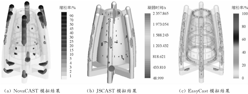
图 5 铸件缩孔缺陷预测 Fig.5 Casting shrinkage defect location prediction
