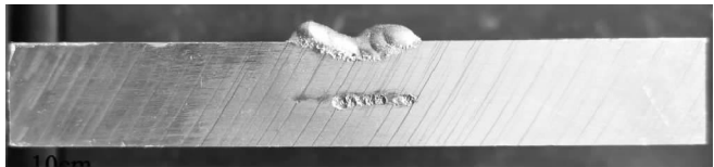
图 5 激光沉积修复试样的形貌 Fig.5 Morphology of laser deposition repairing specimen
