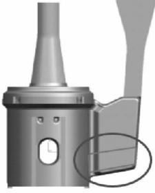
图 8 浇注方案 2 Fig.8 Runner scheme 2
