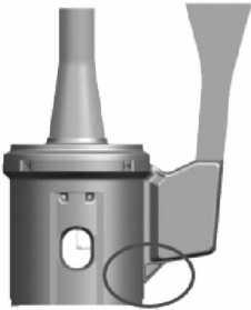
图 7 浇注方案 1 Fig.7 Runner scheme 1
