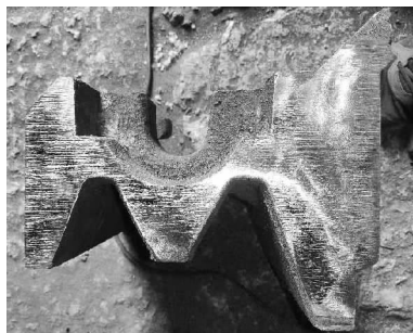
图 10 槽帮铸件冒口附近剖面图 Fig.10 Profile of rump pan casting near the riser
